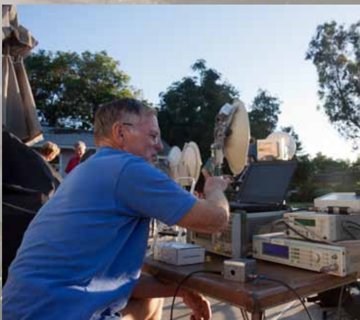
Kerry N6IZW runs the two tests for the range party. Minimum discernible signal and measured output power are recorded for each station. This is a great checkup before the contest season.
