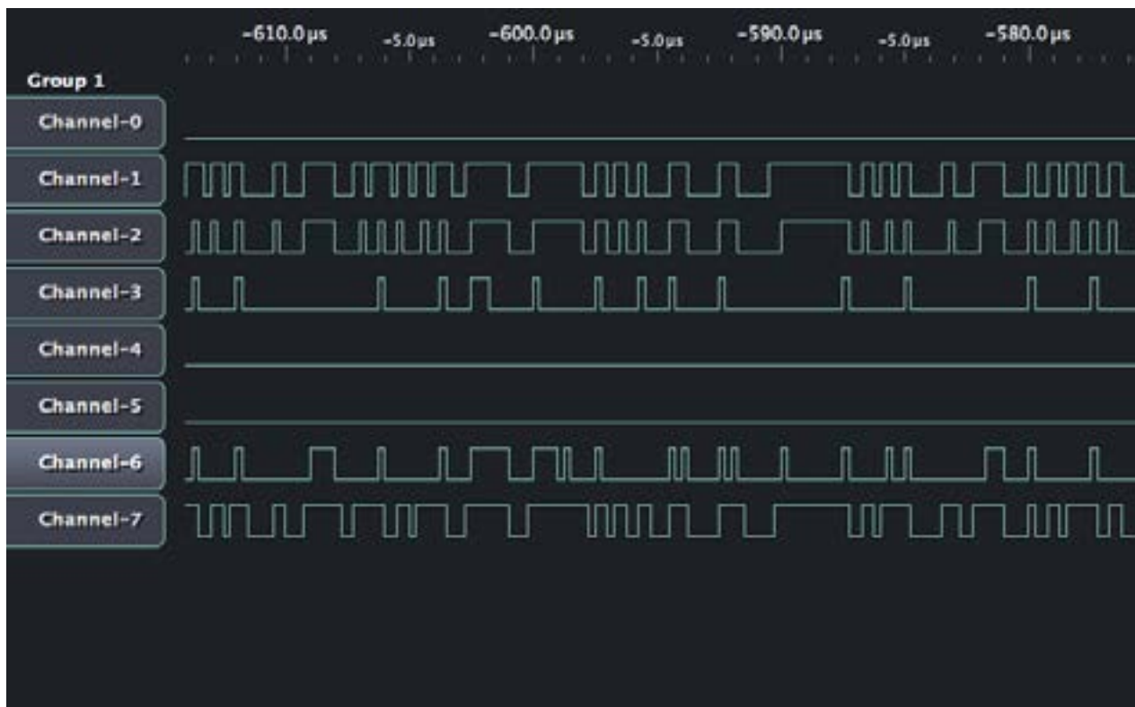
Figure 15: Data from Pin 2 and 3 During Shutter Press
