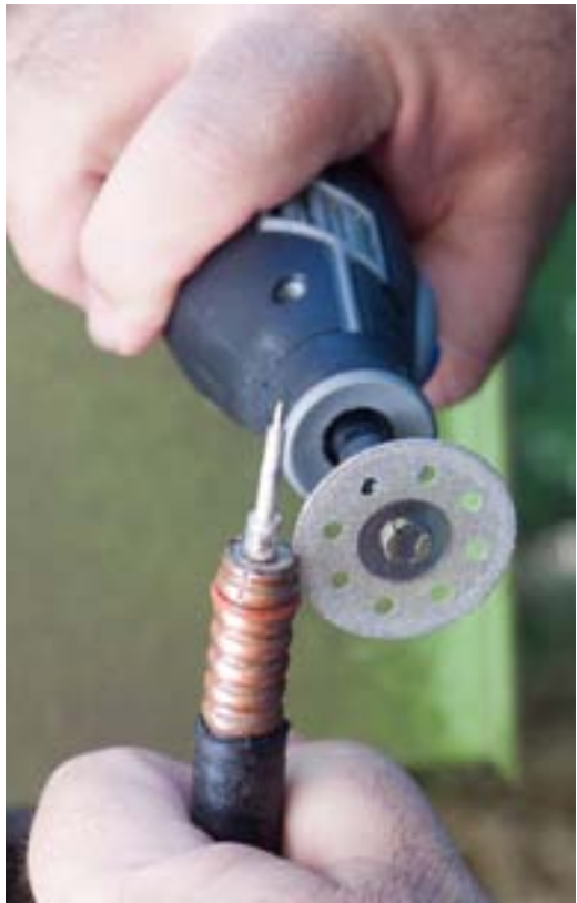
Small cuts to spread the connector collar.
