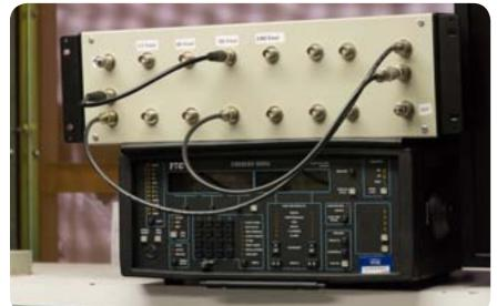
On top, a box of coax loss. On the bottom, a communications analyzer (bit error rate tester and more).
