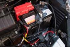
where to find a convenient grommet with room for a big power cable. You have to disassemble the air box (two screws) to see it from the engine compartment. From inside, it's way up under the dash above the gas pedal, but reachable. I cut a slit in it with a Xacto knife and fished my power cable through with a wire coat hanger.
