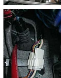
I terminated the power cable near the radio with a standard Anderson Powerpole connector, and constructed a short jumper from Powerpole to the new-style Icom 4-pin power connector, which I found at QSRadio. com. With Powerpoles here I can easily add a RigRunner to provide power for accessories, or power the radio from a separate portable battery or AC power supply. The Fit's own battery is pretty tiny, so I won't be able to operate parked for very long without an auxiliary power source.
