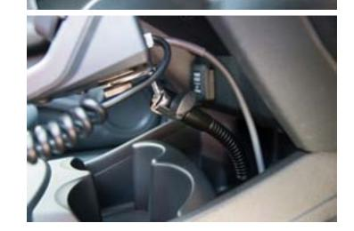
attach to the floor of the square trav instead, which is part of the main console covering. It took only one screw and two plastic push-in fasteners to release the console cover, but I had to unscrew the shifter knob to remove it entirely.
