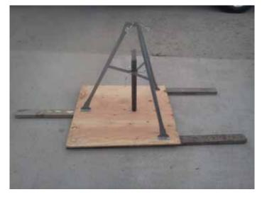
Closeup of new fold over antenna base.
