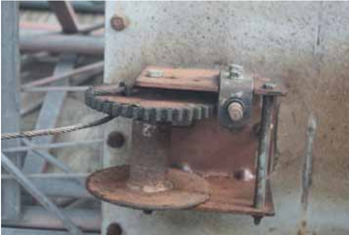
ONE OF THE TWO WINCHES OF CONCERN WITH NO LOCK PAWL.
