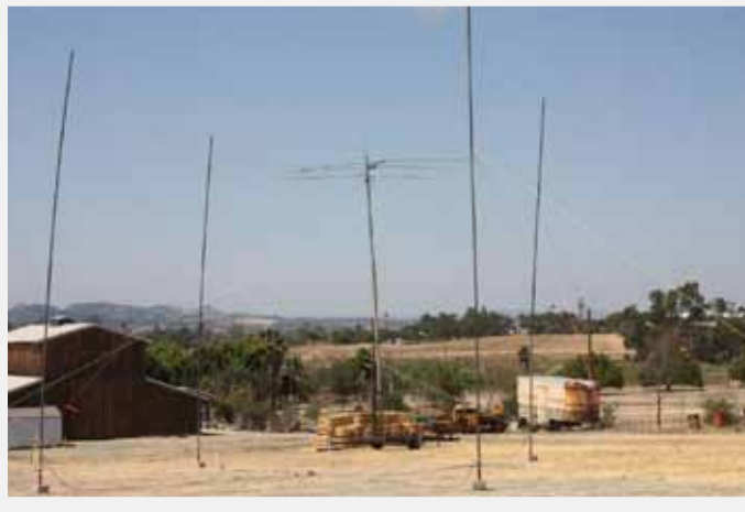
Above, the 40m Four-Square antenna at the 3905 Century Club annual meeting. Below is the 80m in-phase antenna. Photos provided by Loren AD6ZJ.
