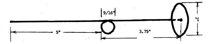
The antenna is made of \$14 hard drawn copper wire. The coil is 5 1/4 turns, 9/16" diameter. Top hat is 2" diameter of thin copper or tin. Solder the antenna into whichever type connector fits your HT. This antenna provides 6db gain over a rubber ducky - so we hear. Thanks to Max for the foregoing. He says he has seen measurable gain with this contraption.
