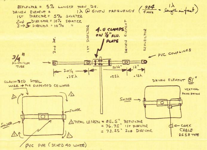
The antenna is made from  $\frac{1}{2}$ " aluminum tubing and PVC pipe fittings. The elements are 1/8" galvanized steel wire of the type used to suspend ceilings, which is usually available at the larger building supply stores.
