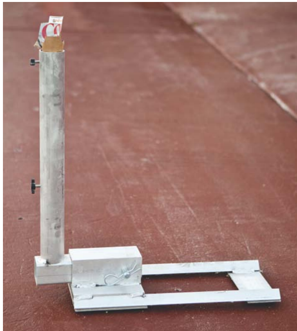
The base is in two parts: the horizontal platform provides a standard 2" trailer hitch receiver, and the vertical tubing is welded to a square tube that fits inside it. The cardboard you can see sticking out of the vertical tube (from a 12-pack of Coke) is to protect the surface of the telescoping mast from being damaged by the screws in the base.
