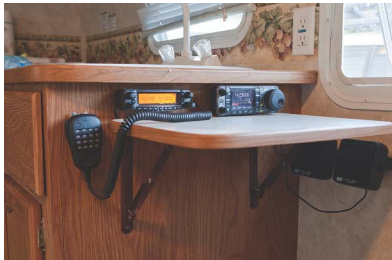
Yes, the IC-7000 can also do VHF and UHF, but I wanted to be able to monitor VHF and UHF FM continuously while also tuning around on HF. A separate VHF/UHF rig makes this possible. The FT-8900R also supports 6m and 10m; these bands don't add much to the price and might come in handy someday.
