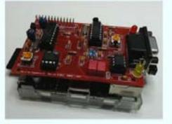
The original TNC-Pi sits atop Raspberry Pi version 8. The 9 pin D-sub connector interfaces to your radio.
