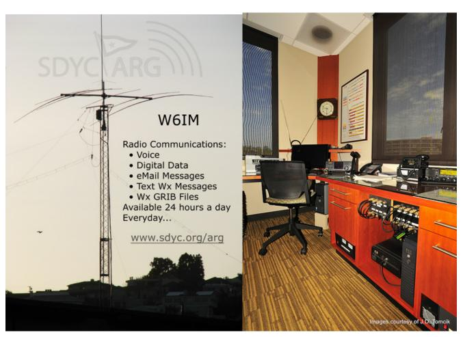
Under the North window, is a Marine Communication Station consisting of an ICom IC-M710 HF (1.8 MHz - 30 MHz) Marine Single Side Band (SSB) radio and an ICom IC-M59 Marine VHF (156.00 MHz - 163 MHz).
