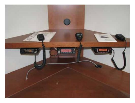
The VHF/UHF station includes a Kenwood TM-221A (144 MHz - 148 MHz) 2 Meter VHF radio. In the center is an Alinco DR-235 (222 MHz - 225 MHz) 1.25 Meter VHF radio. Also included is a Yaesu FT-7900R multiband VHF/UHF radio for 2 meters and 70 centimeters.
