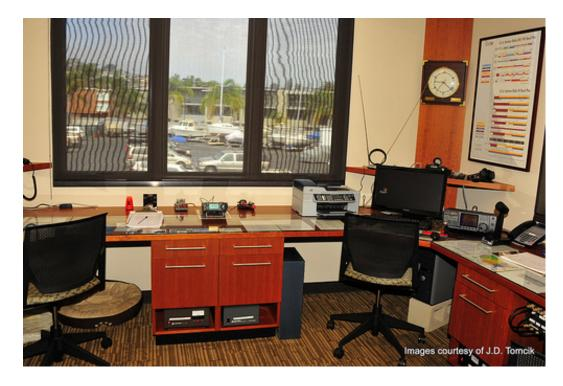
The radio room was designed to be neat and efficient with HF, UHF/VHF and WinLink operating positions. Desks and paneling were selected to match and cable runs were concealed.
