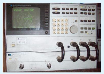
This is a Hewlett-Packard 3577A with the 35677A S-Parameter test set and all interconnect cables.
