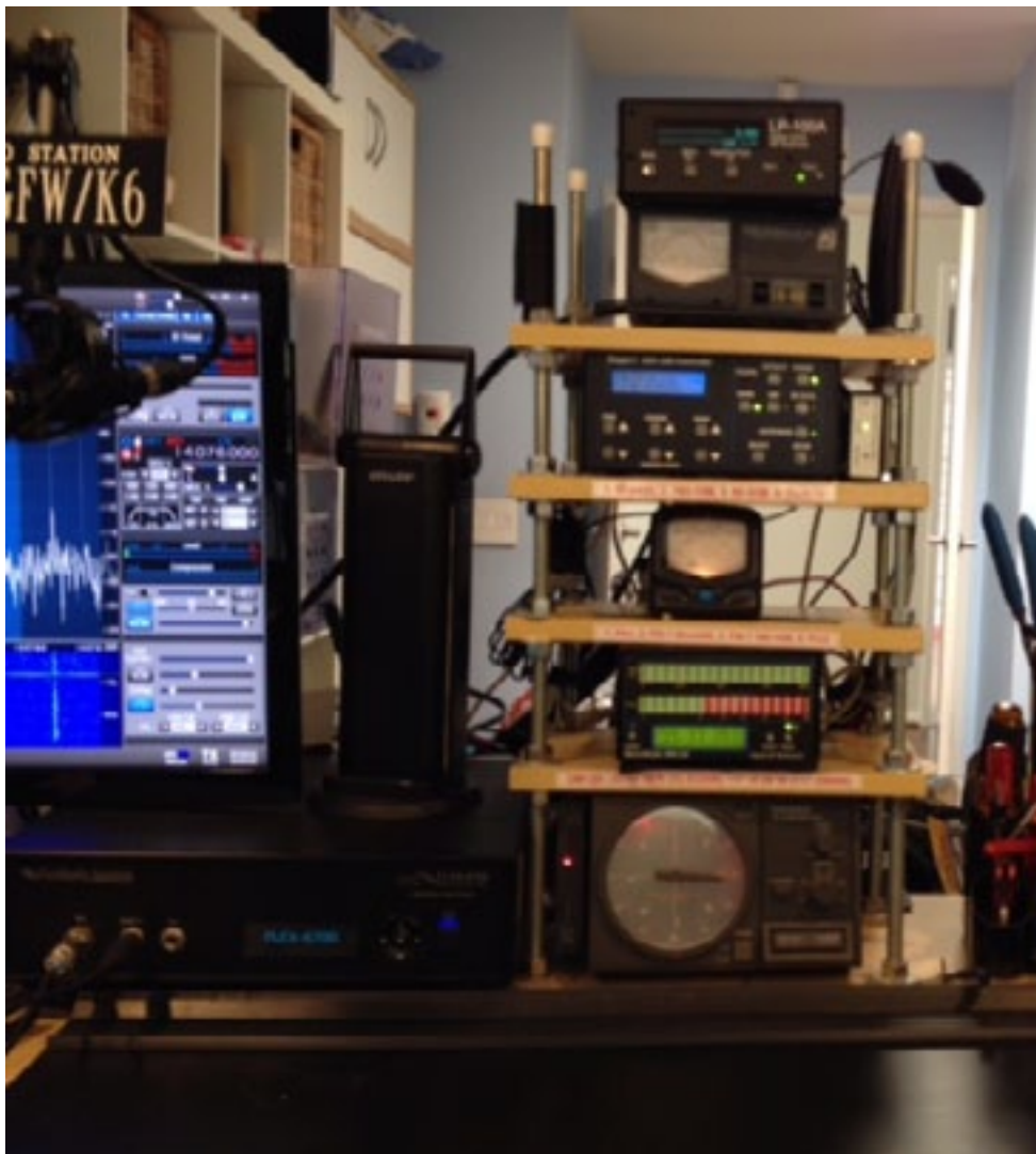
This is a 2' -4shelf X 1' stack for rotor:controls, SteppIR controls and 4 wattmeters.
