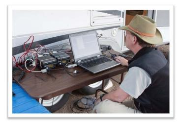
Above, Dean K6DBJ mans the central database station. Two transceivers and two TNCs are used to accommodate simplex users a separate channel from digipeater users.
