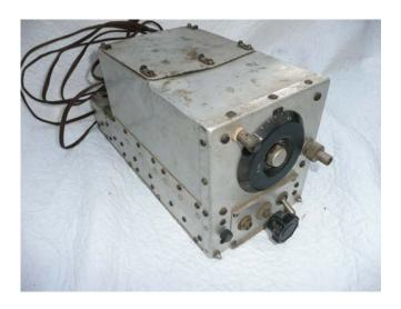
Other popular models covered 1.5 to 3 and 3 to 6 MHz. The aircraft had 24 volt electrical systems, so the filaments were wired in series/parallel for that voltage. Most users rewired the filaments. Also, a small power supply had to be built to provide the high voltage that was supplied by a dynamotor in the airplanes.
