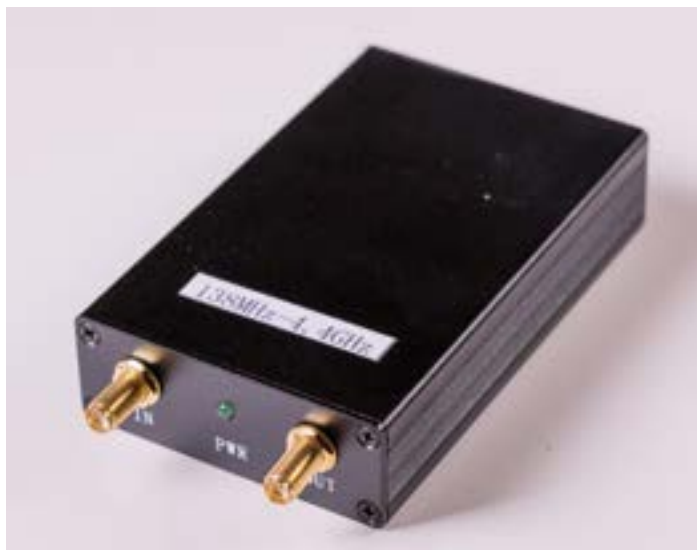
The BG7TBL signal generator and spectrum analyzer device.
