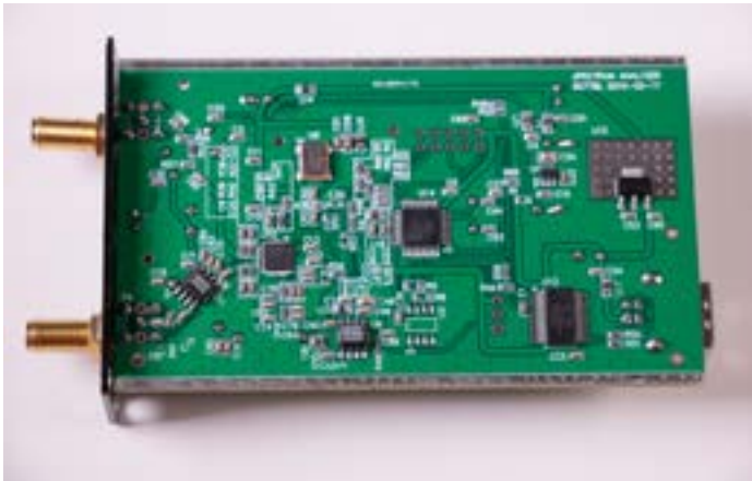
The BG7TBL signal generator and spectrum analyzer device, bottom of circuit board.
