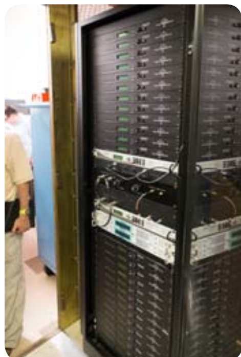
This rack of equipment simulates a DirecTV satellite system for receiver testing.
