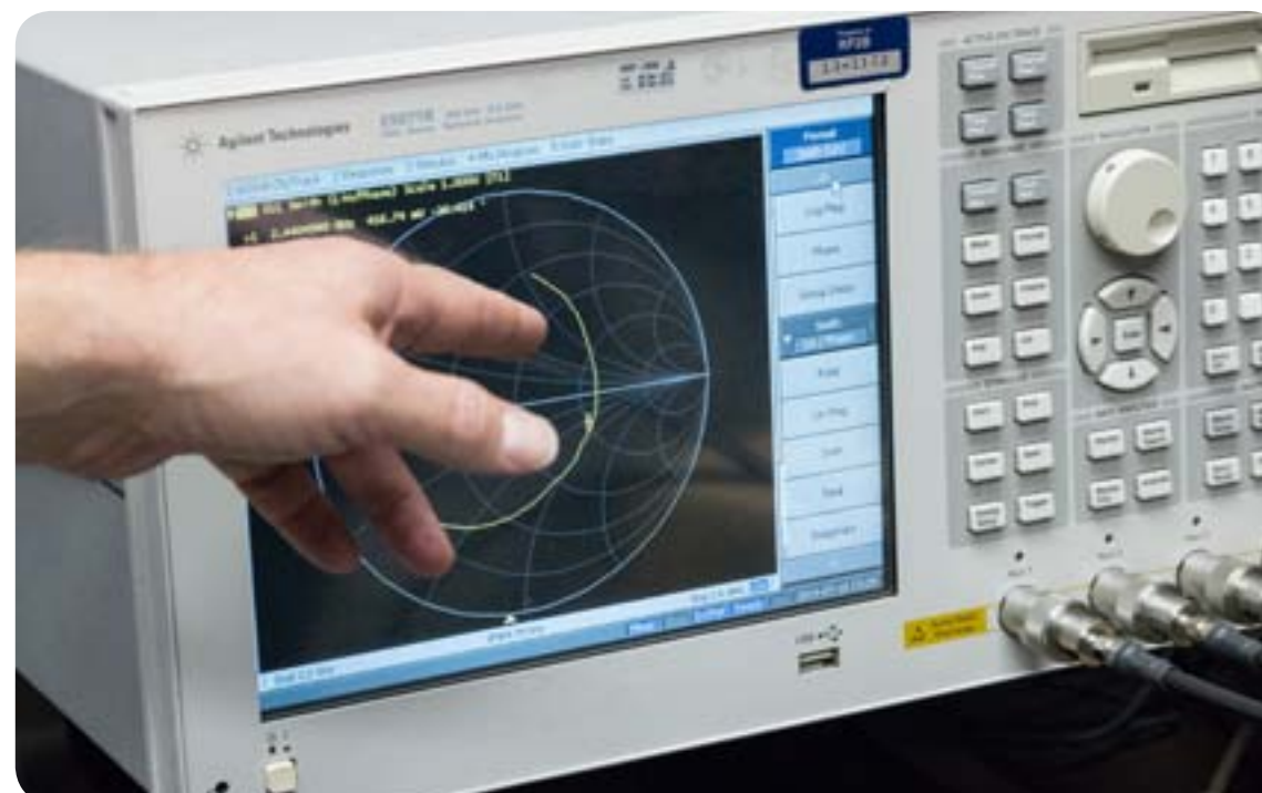
Mats AG6CV explains the Smith Chart display mode of the network analyzer.
