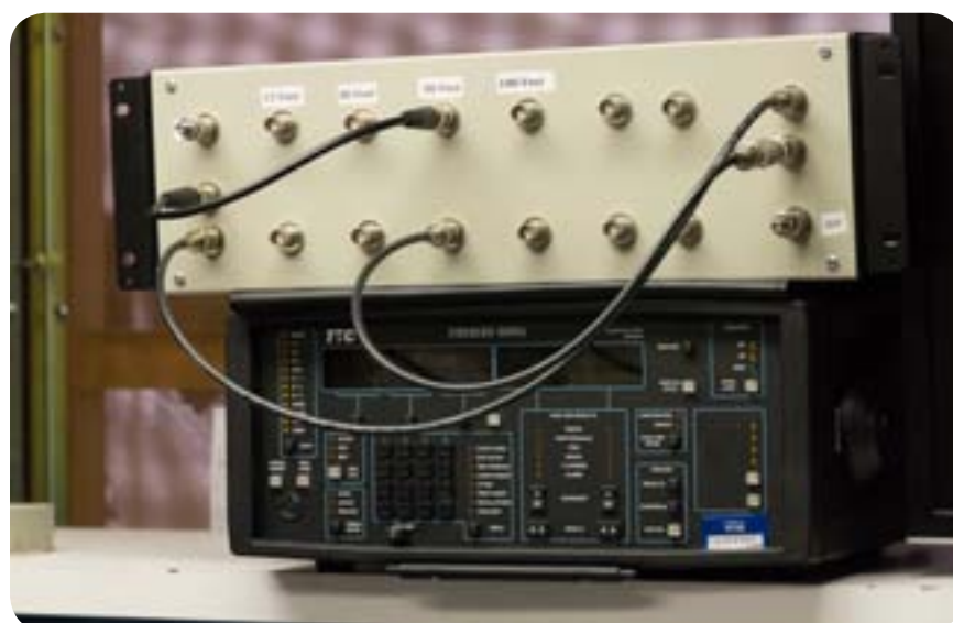
On top, a box of coax loss. On the bottom, a communications analyzer (bit error rate tester and more).
