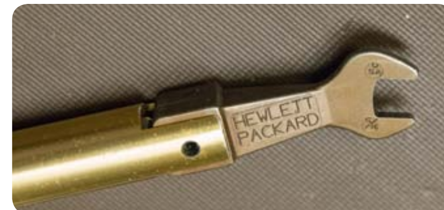
This is a dedicated 5/16" torque wrench specifically for tightening SMA connectors.
