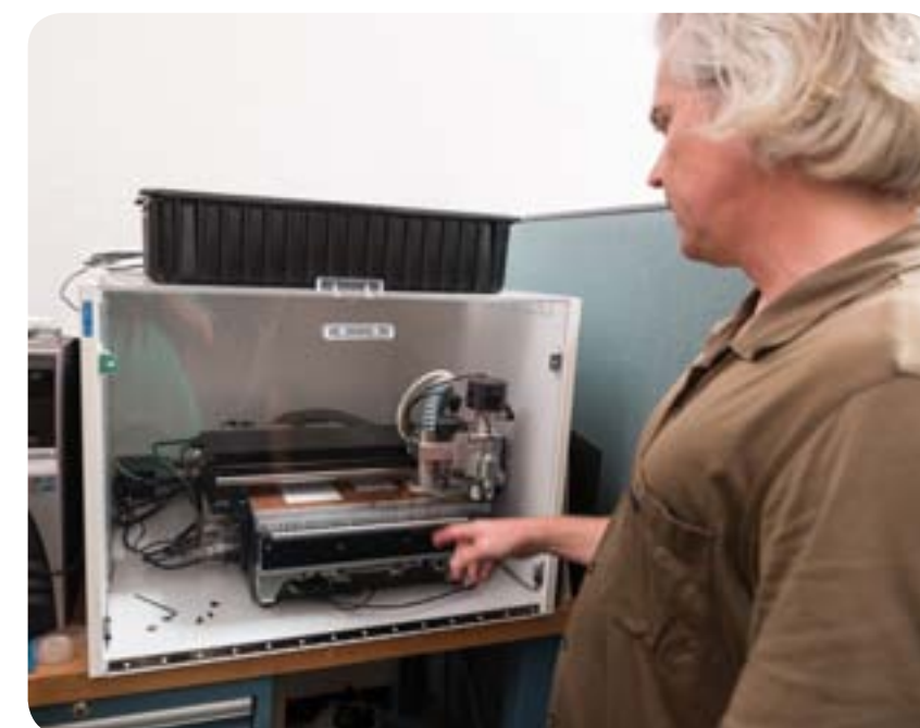
Mats AG6CV describes the CNC router (with automatic tool changer) for making prototype circuit boards.
