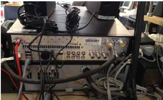
Installation was a breeze. Open box, plug in antenna, GPS antenna, microphone, speakers, Ethernet cable. Connected a 12V power supply, downloaded the SmartSDR Preview Beta Test Software (V0.12.17). It installed automatically. Firmware was updated on the radio, and Voila, I was on the air.
