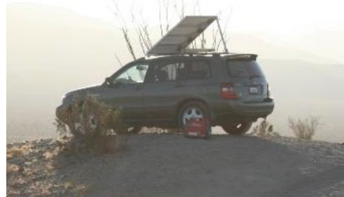
KF6NXY's solar panels supplying cross band repeater.
