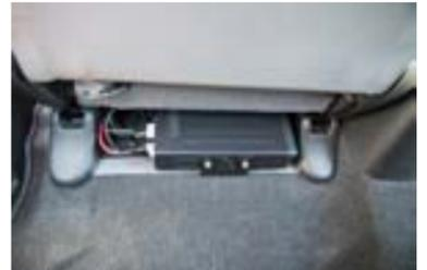
One problem with this location is that the heating vent for the rear passenger blows directly at the radio. I'm just hoping this won't cause an overheated radio or a grumpy frozen passenger.
