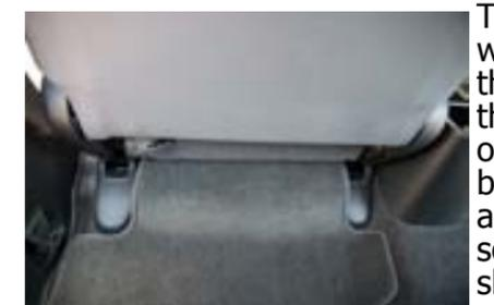
The next question was how to mount the radio unit there. It has vents on the top and bottom as well as at both ends, so it probably should not be placed directly on the carpet. The IC-7100 does not come with a mounting bracket for the main unit (boo, Icom), but the MB-62 bracket is available. What I've done in the past is cut two slits in the carpet for the vertical ears of the mounting bracket, so I
