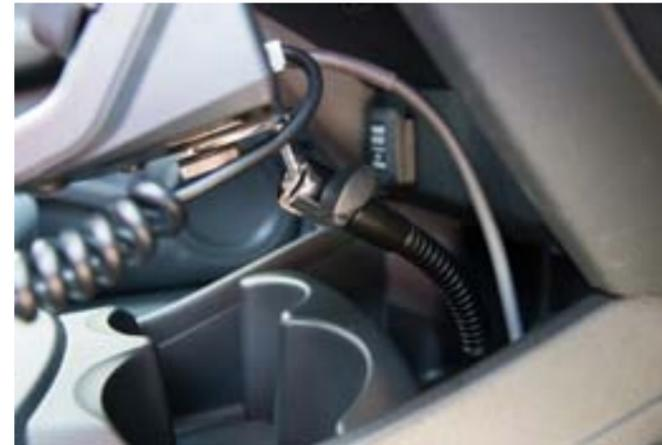
attach to the floor of the square tray instead, which is part of the main console covering. It took only one screw and two plastic push-in fasteners to release the console cover, but I had to unscrew the shifter knob to remove it entirely.
