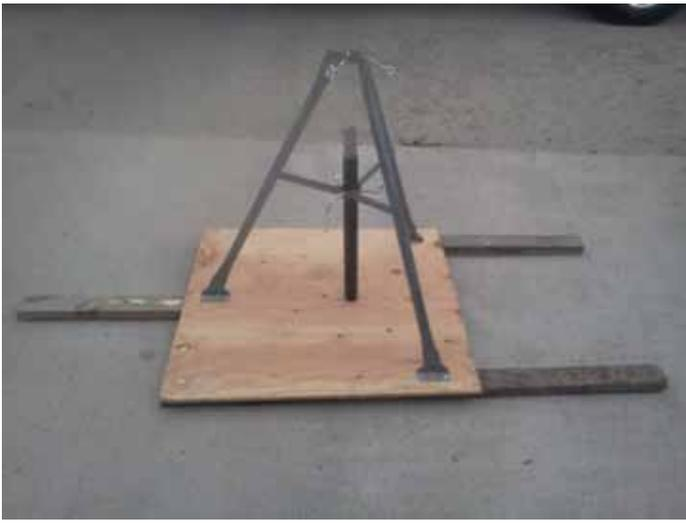
Closeup of new fold over antenna base.
